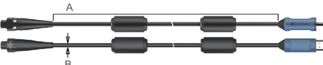
The diagram shows two parallel views of the cable. The top view shows the full length of the cable with a dimension line labeled 'A' indicating the total length. The bottom view shows a cross-section of the cable with a dimension line labeled 'B' indicating the diameter.
