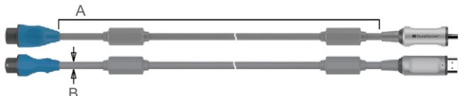
The diagram shows two parallel cables. A horizontal line labeled 'A' spans the length of the top cable. A vertical double-headed arrow labeled 'B' indicates the diameter of the cable.
